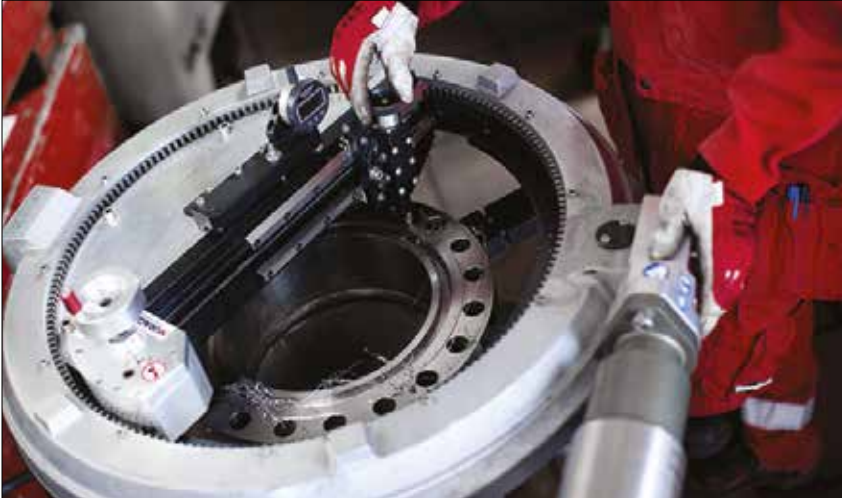
▲ Flange facing machining.
