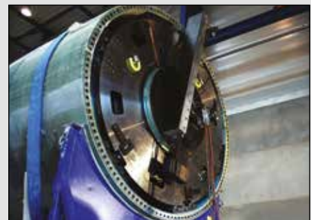
▲ Orbital milling machines for wind turbine manufacture.
