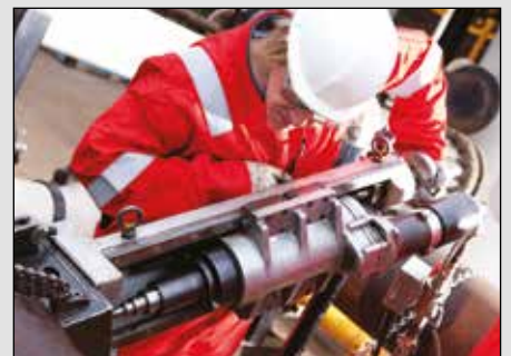
▲ High torque portable drilling machines.
