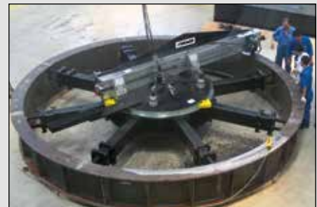
▲ Orbital milling machines used in shipbuilding and power generation industries.
