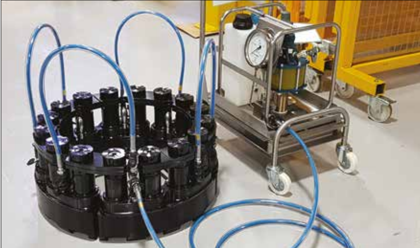
▲ Multi Stud Tensioning Set-Up.
