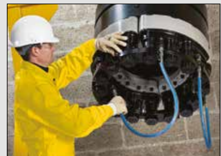
▲ Multi Stud Tensioning application.
