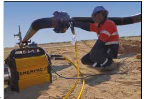
E-Pulse torque pump used for high volume fastening applications where weight is a critical factor. ▶
