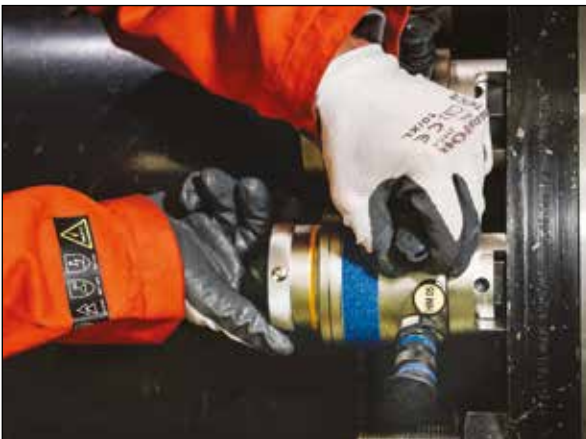
◀ Enerpac HM-Series HydraMax® tensioners have been designed to generate high bolt loads associated with compact flanges, while providing versatility for maximum bolt coverage,
