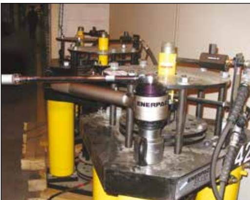
◀ Enerpac Reaction Bar Torque Multiplier E393 used to manually torque bolts up to 4300 Nm.
