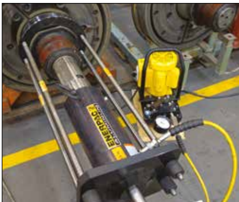
◀ Rail wheel pulling with RACH-cylinder and ZE-Series electric pump.
