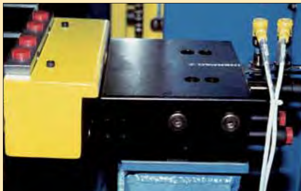
■ A 4-way auto coupler is connected to the receiver, mounted on the side of a palletized fixture.
