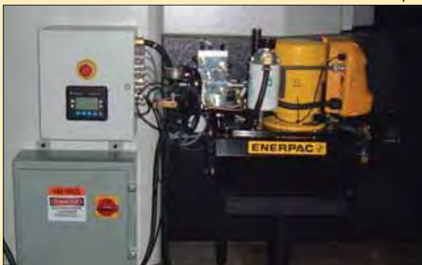
■ ACCB-2 Control shown with ZW4020HJ-FHLT12U300 Pump.
